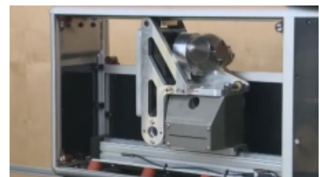
A Fredericton engineering company has developed technology it describes as a culvert ‘cat scan’ to inspect tunnels.
